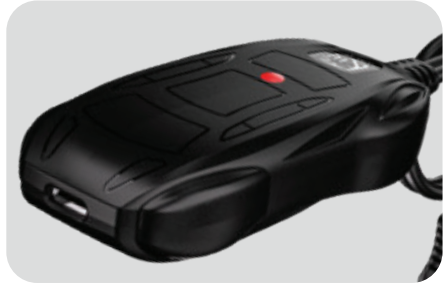
4. Solid Red (Check connections are correct / Check battery is below 3V)
